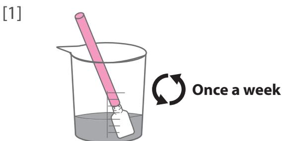
Prepare another cleaning stick to clean the cleaning wiper and around the capping unit.
